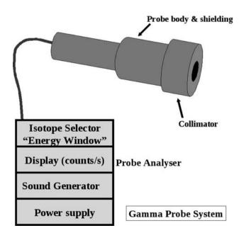
FIG. 2 Components of the gamma probe
